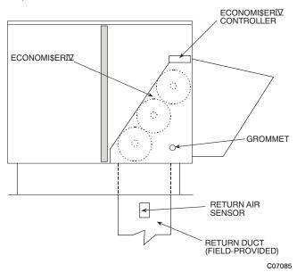
Fig. 79 - Return Air Temperature or Enthalpy Sensor Mounting Location
